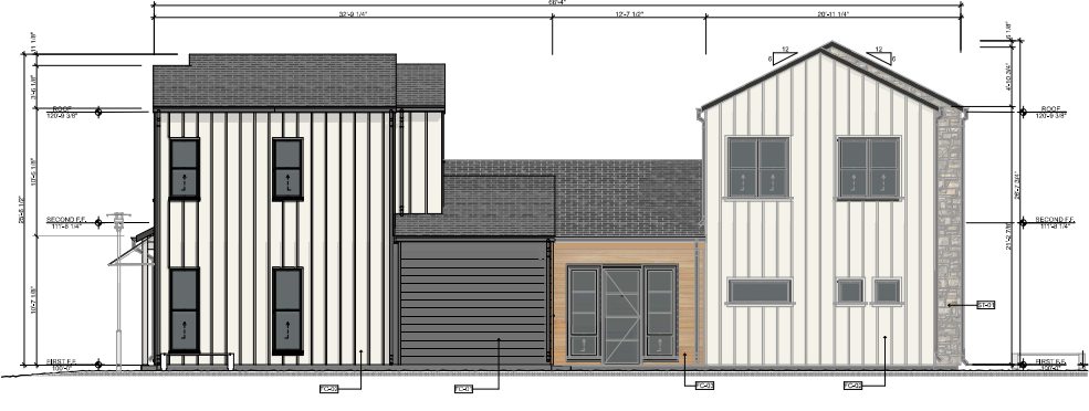
3 COURTYARD SOUTH ELEVATION - B2&C1 (REAR) SCALE: 3/16" = 1'-0"
