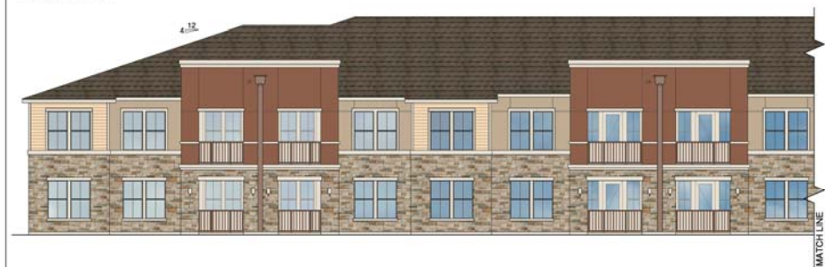
2 BUILDING B - COURTYARD ELEVATION (WEST) SCALE 1/8"=1'-0"
