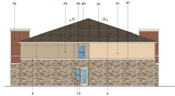
3 BUILDING B - SIDE ELEVATION (NORTH) SCALE 1/8"=1'-0"
