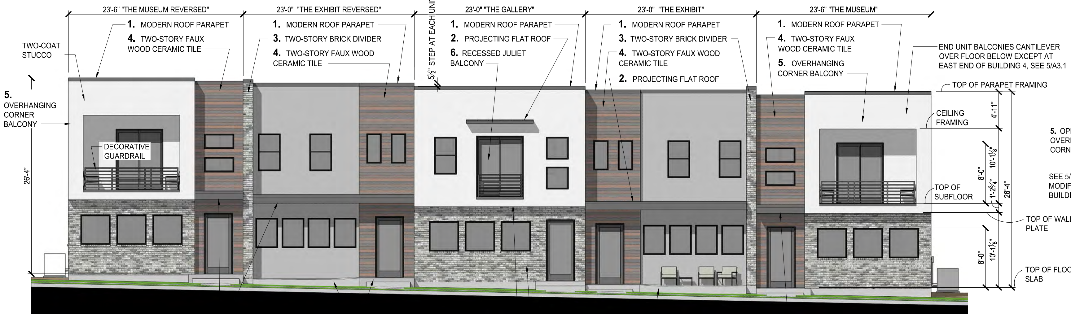
ELEVATION SOUTH/FRONT BUILDINGS 1, 2, 8, & 9
