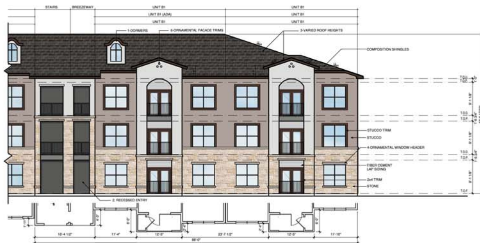
4b BUILDING - COURTYARD WEST ELEVATION SCALE: 1/8" = 1'-0"
