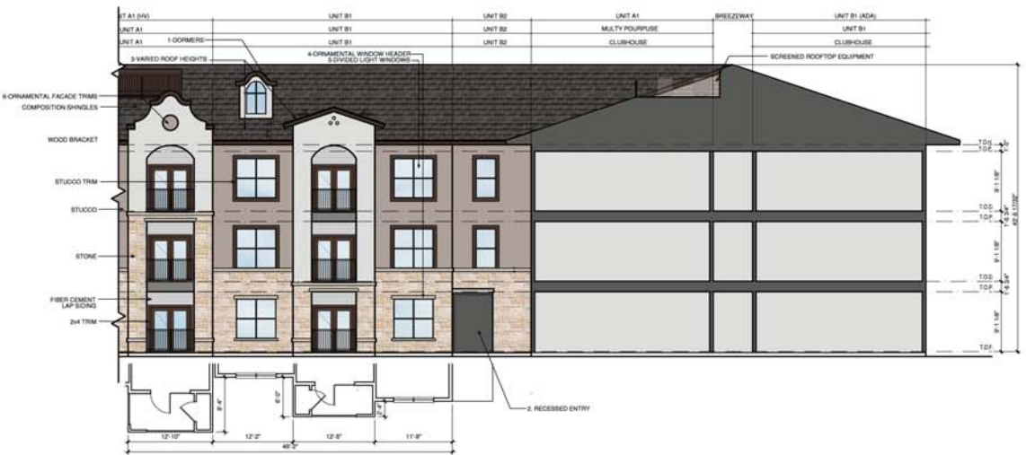
5a BUILDING - COURTYARD EAST ELEVATION SCALE: 1/8" = 1'-0"
