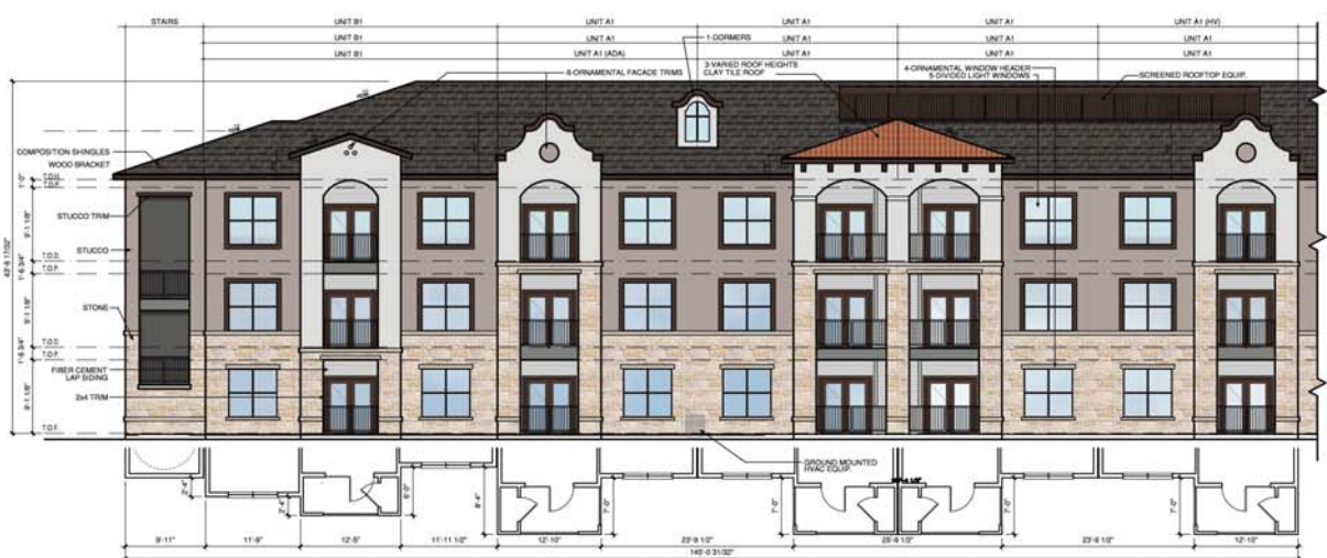
5a BUILDING - COURTYARD EAST ELEVATION SCALE: 1/8" = 1'-0"
