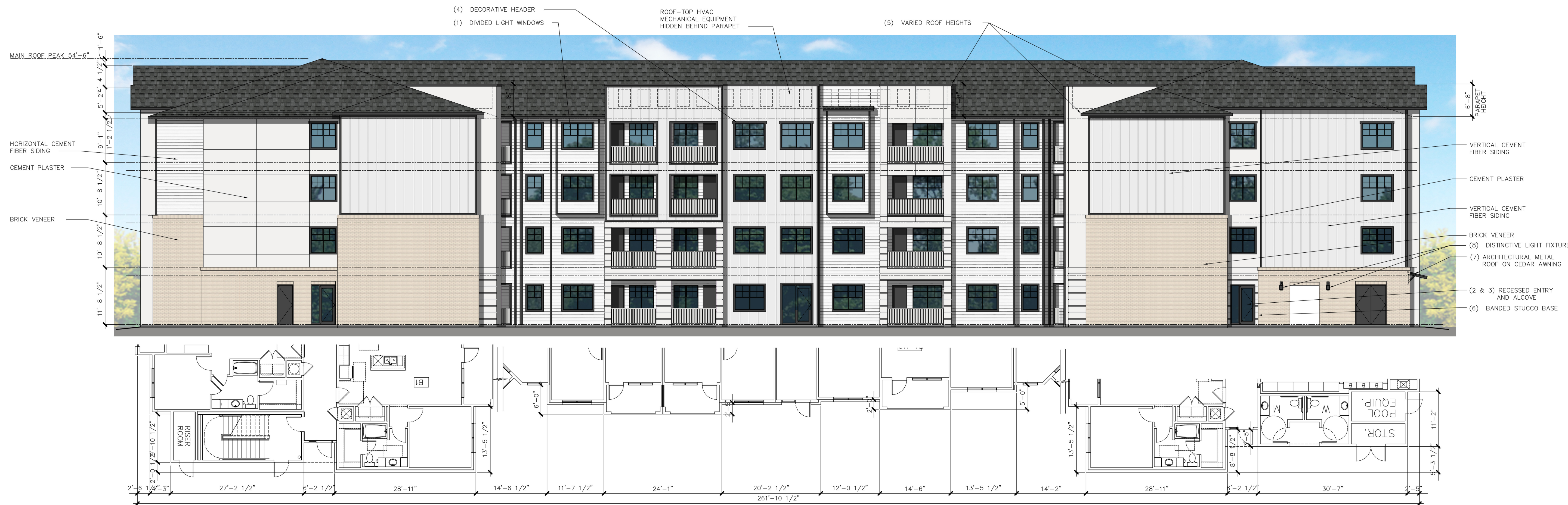
01 BUILDING 1 - NORTH-WEST ELEVATION (POOL AREA VIEW) SCALE: 3/32" = 1'-0"
