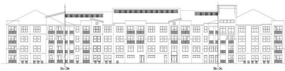
3 BUILDING 'C' SOUTH OVERALL ELEVATION SCALE: 1" = 20'-0"
