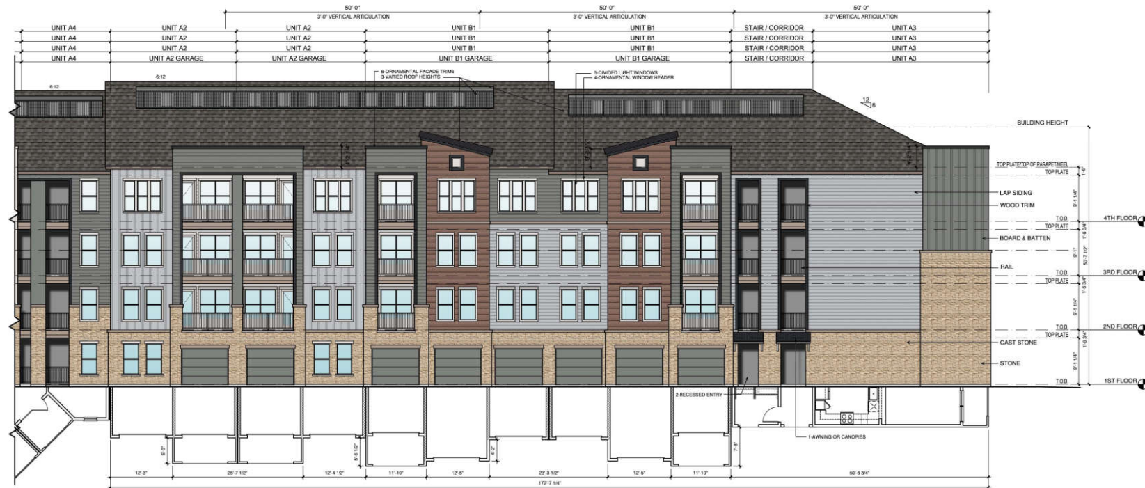
3b BUILDING B - NORTH EXTERIOR ELEVATION SCALE: 1/8" = 1'-0"
