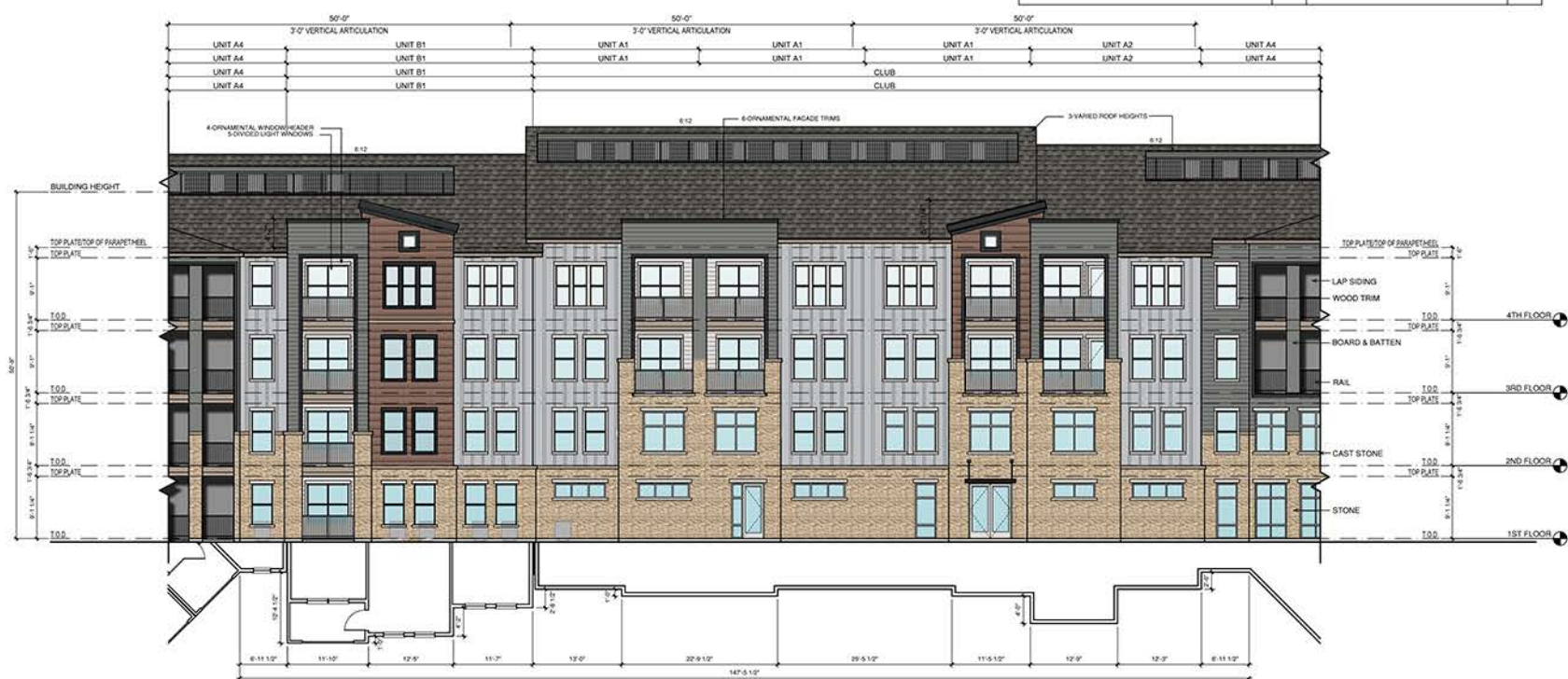
3b BUILDING C - SOUTH EXTERIOR ELEVATION SCALE: 1/8" = 1'-0"
