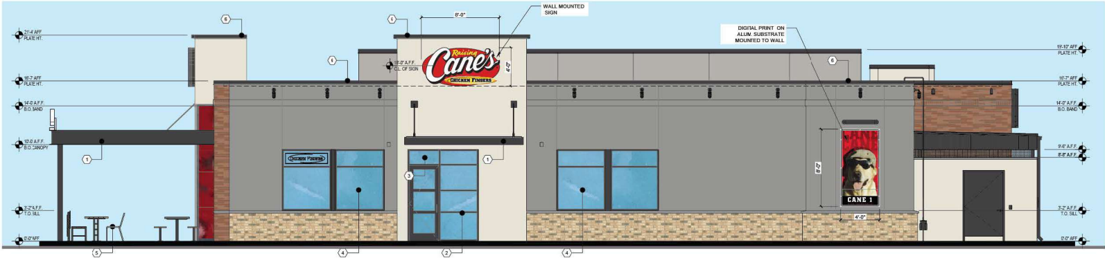
2 | SOUTHWEST ELEVATION (SIDE ENTRY) SCALE: 1/4" = 1'-0"
