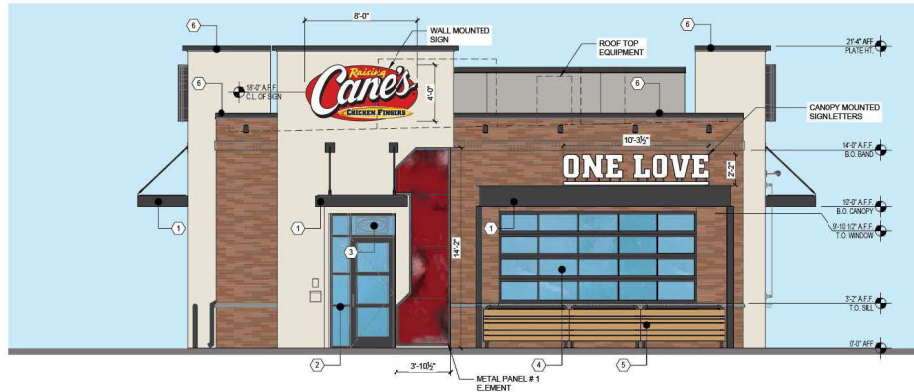
1 | NORTHWEST ELEVATION (FRONT ENTRY) SCALE: 1/8" = 1'-0"
