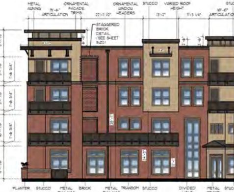
2 EXTERIOR ELEVATION (WEST)
