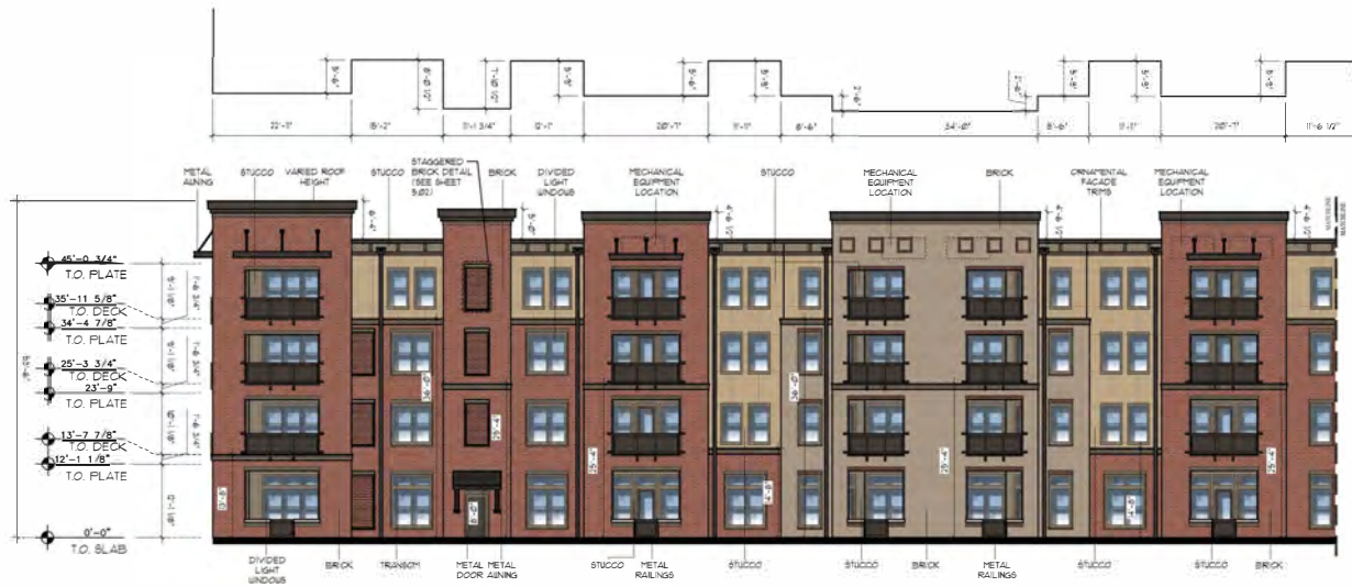
2 EXTERIOR ELEVATION (NORTH) SCALE: 1/8" = 1'-0"
