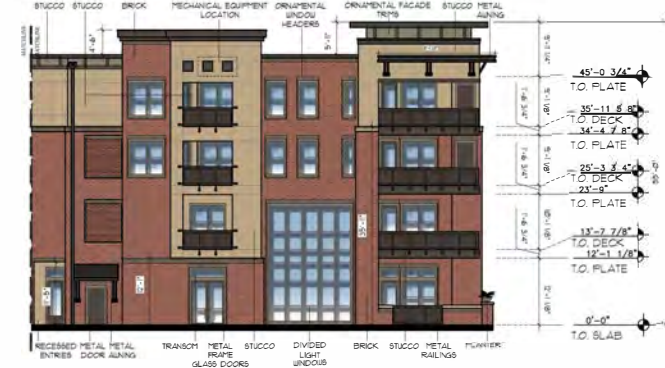
2 EXTERIOR ELEVATION (NORTH) SCALE: 3/8" = 1'-0"
