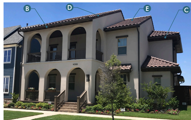
A Shallow eave with stucco profile; B Exposed rafter tails; C Eave brackets; D Rake tile detail; E Barrel tile roof; F Barrel tile gable detail; G Board and batten shutters
