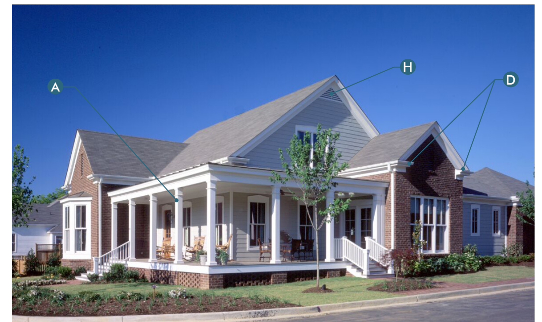
A Prominent front porch; B Bracket detail on rake; C Exposed rafter tails; D Eave returns; E Gable pediment detail; F Shed dormer; G Stone accent on chimney; H Gable vents or windows
