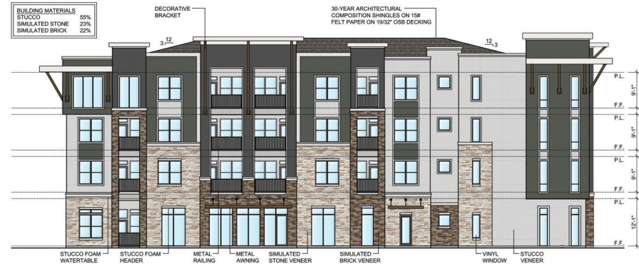
01 BUILDING 'A' - NORTH ELEVATION SCALE: 3/32" = 1'-0"
