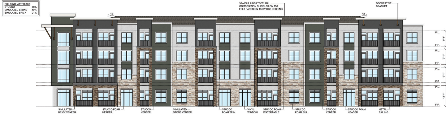
03 BUILDING 'A' - EAST ELEVATION SCALE: 3/32" = 1'-0"
