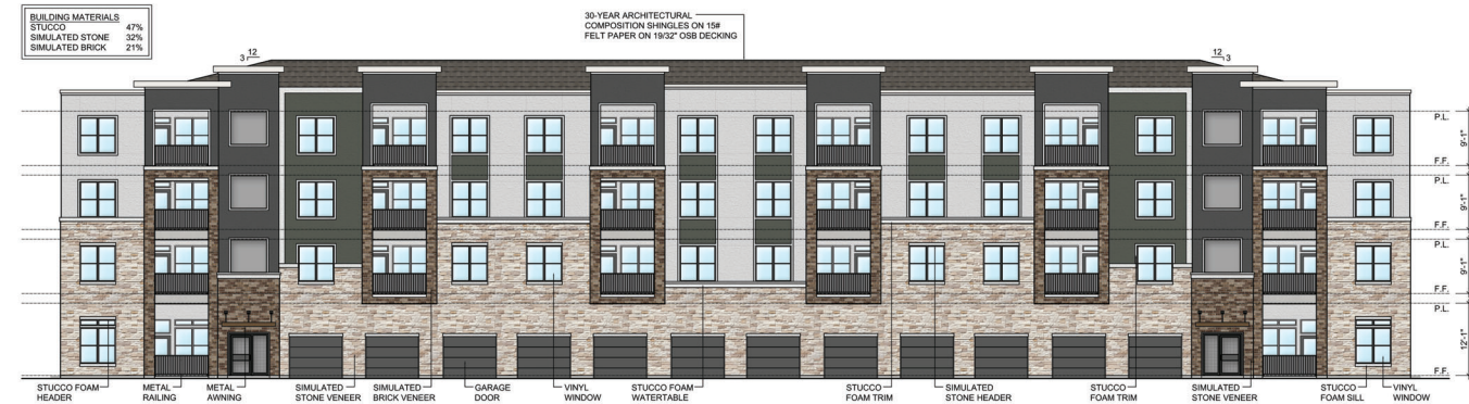
01 BUILDING 'B' - NORTH ELEVATION SCALE: 3/32" = 1'-0"
