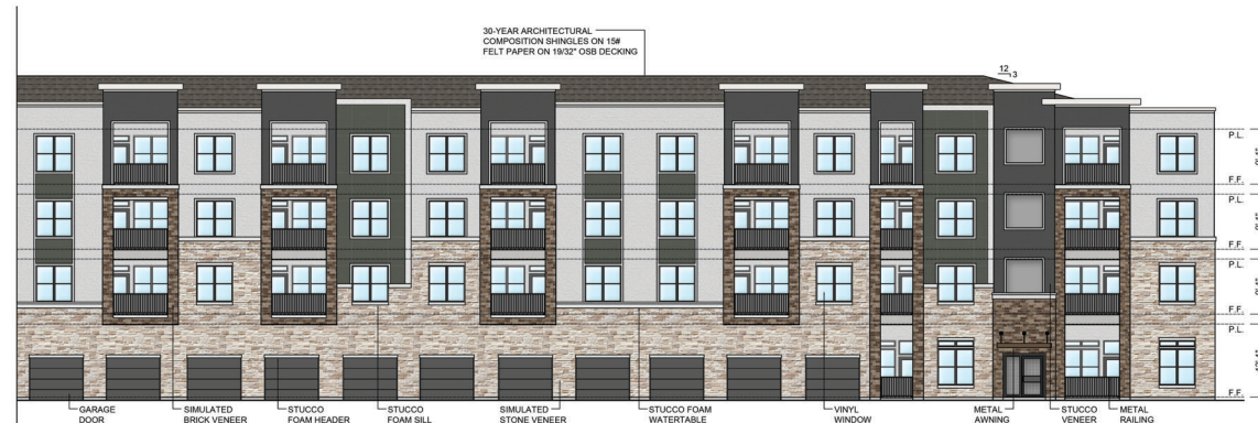
01 BUILDING 'E' - NORTH ELEVATION SCALE: 3/32" = 1'-0"
