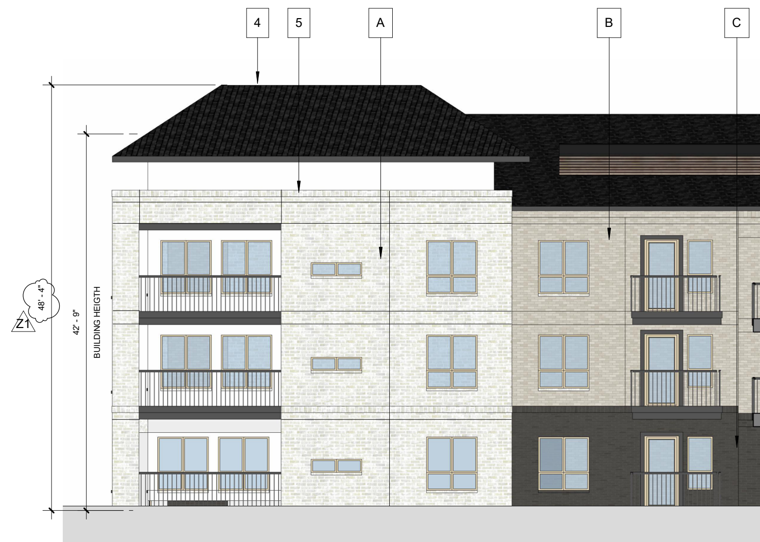
20 BUILDING 3 - WEST ELEVATION 3/32" = 1'-0"
