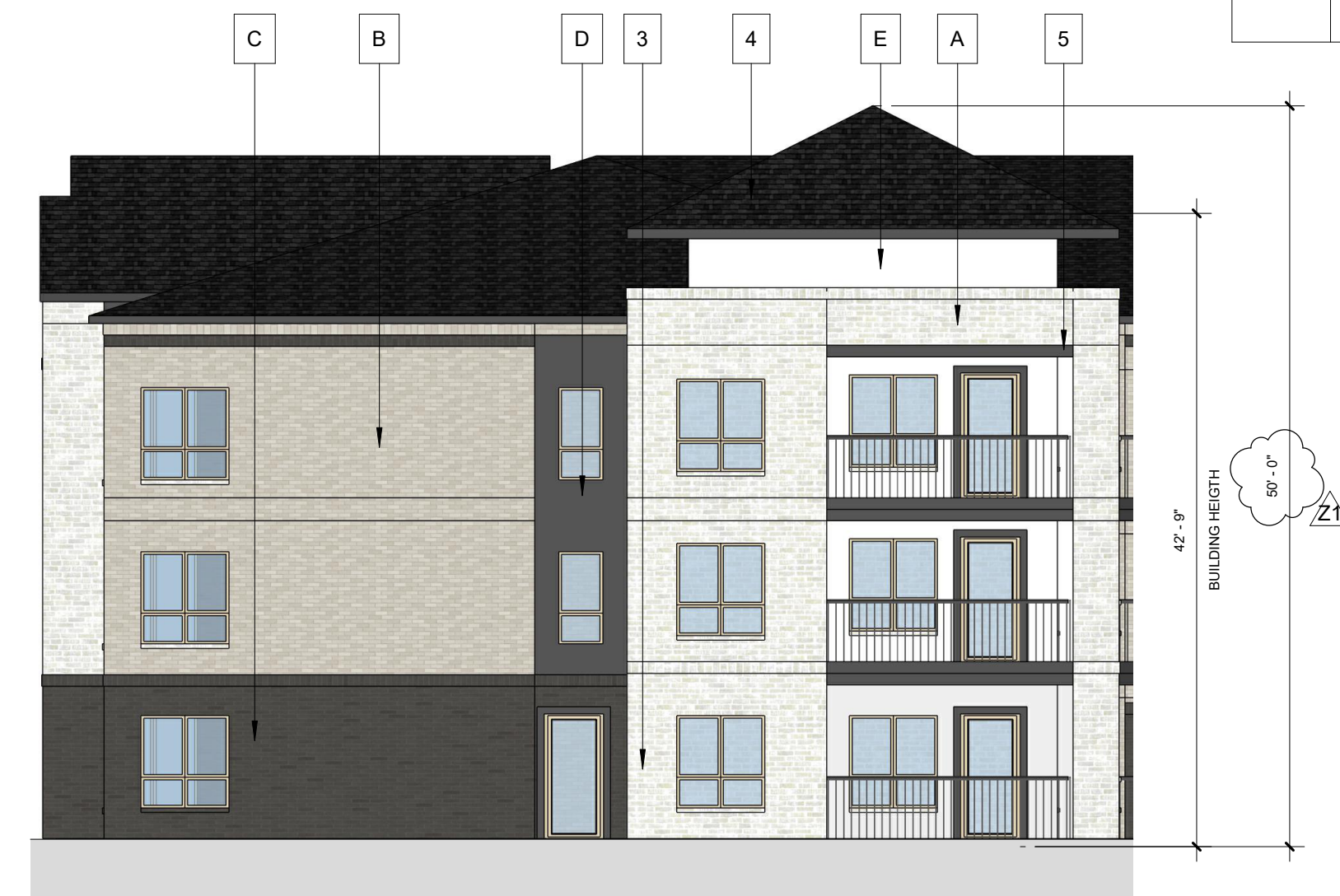
19 BUILDING 3 - NORTH ELEVATION 3/32" = 1'-0"
