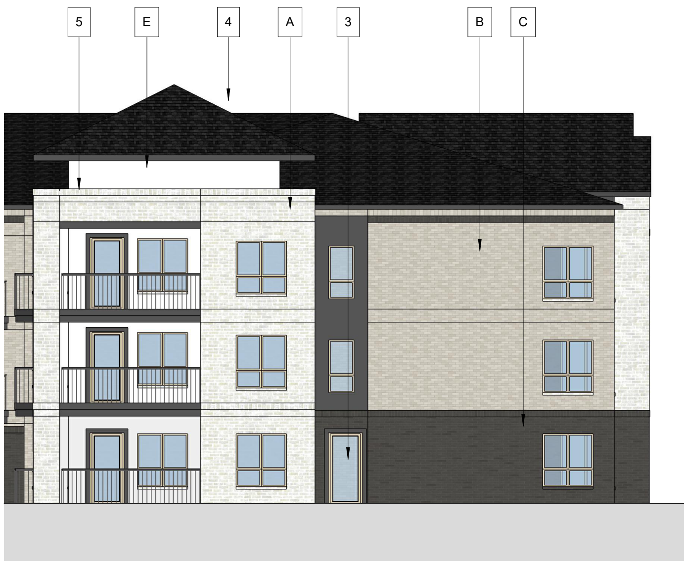
23 BUILDING 3 - NORTH ELEVATION 3/32" = 1'-0"
