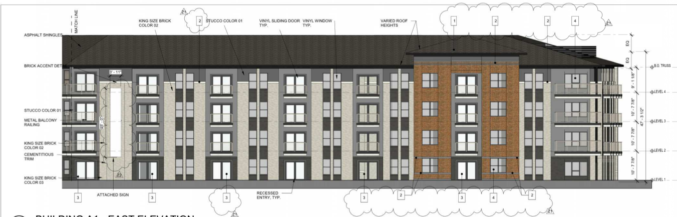
BUILDING A1 - EAST ELEVATION 3/32" = 1'-0"
