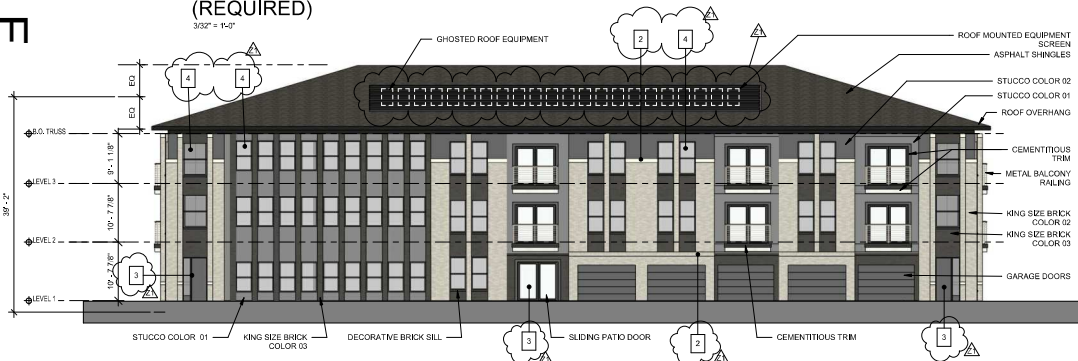
BUILDING ARTICULATION FACING STREET (REQUIRED) 3/32" = 1'-0"
