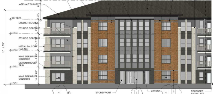
BUILDING A1 - SOUTH-EAST ELEVATION 3/32" = 1'-0"
