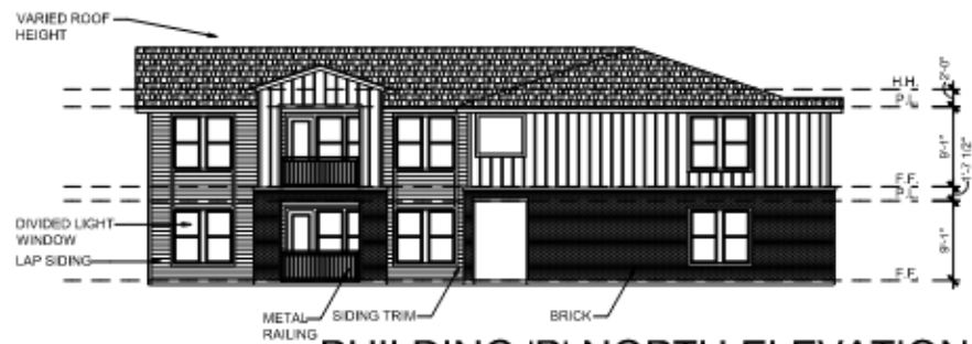
BUILDING 'B' NORTH ELEVATION SCALE: 1/16" = 1'-0" 1 REQ. @ BLDG #2
