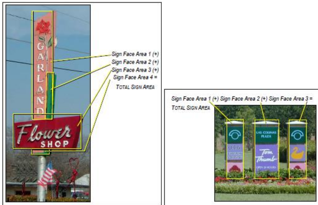
Illustration 4-5 Sign Area - Irregularly Shaped Signs
