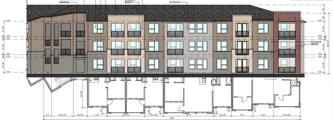
2 BUILDING TYPE 'B' FRONT ELEVATION
