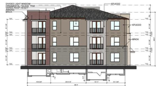
2 BUILDING TYPE 'D' END ELEVATION
