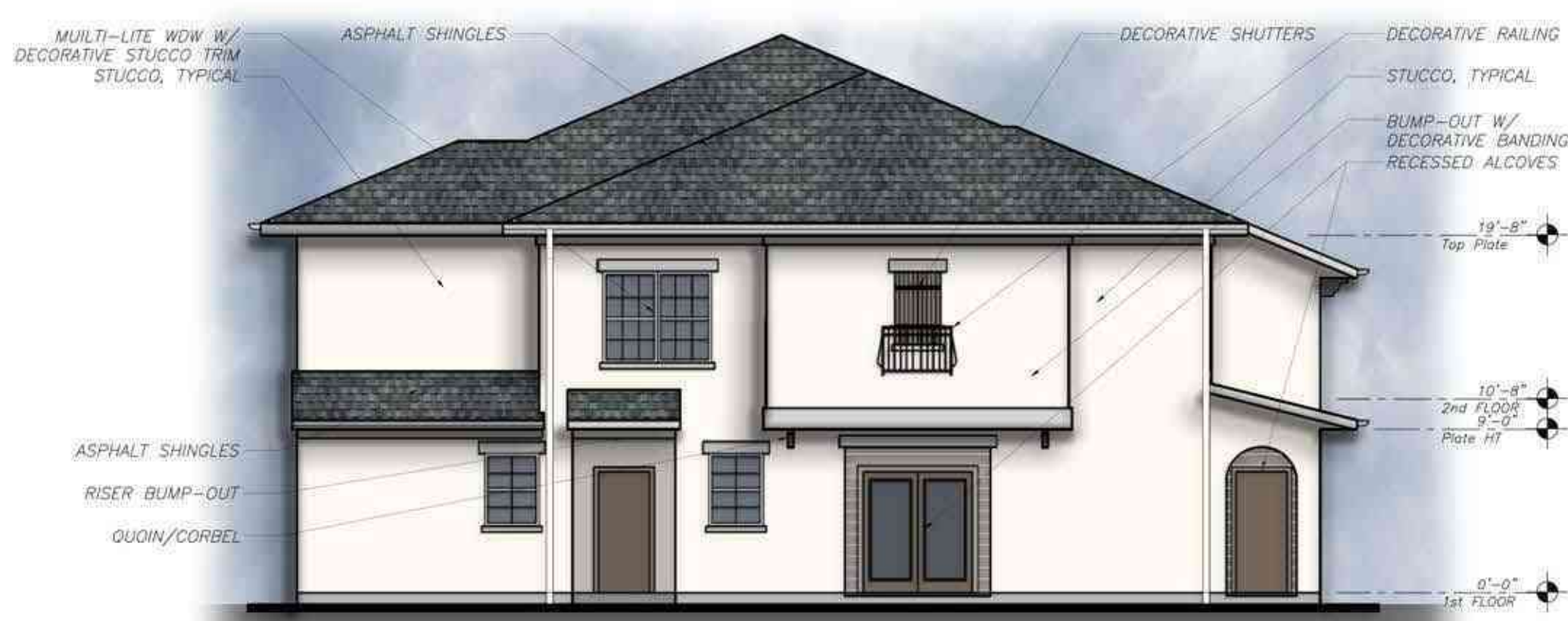
04 TYPE 4 - LEFT (NOM. WEST) ELEVATION
