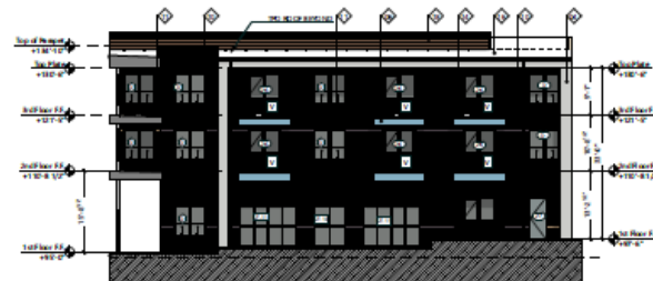
25 Building 1 Courtyard East Elevation Scale: 1/8" = 1'-0"
