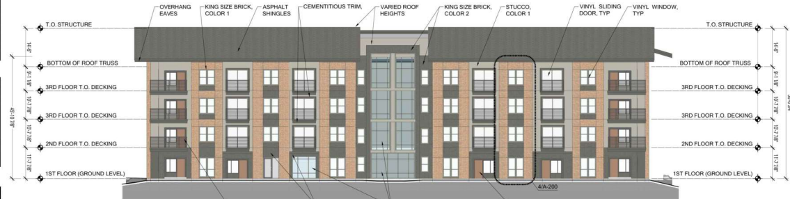
03 BUILDING 1 - WEST ELEVATION (XREF: SD-Elevations.dwg) Scale: 1/16" = 1'-0"
