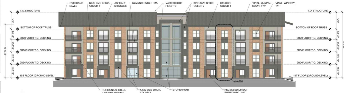
03 BUILDING 1 - WEST ELEVATION (XREF: SD-Elevations.dwg) Scale: 1/16" = 1'-0"
