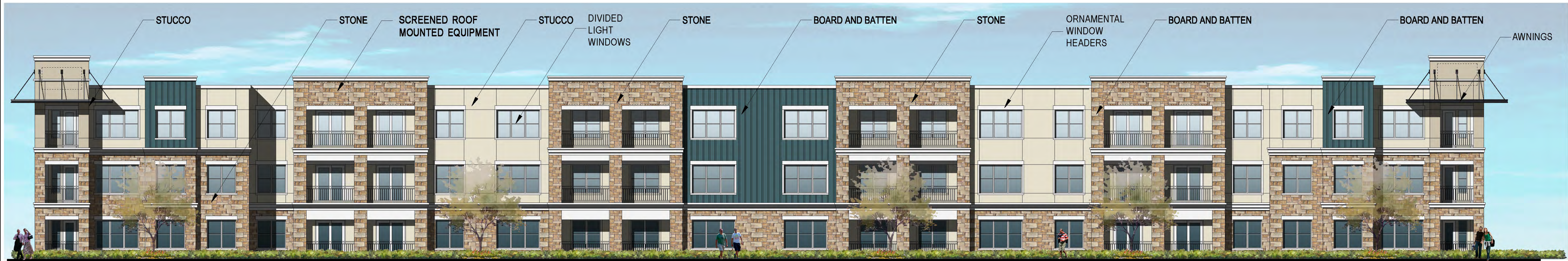
REAR ELEVATION BUILDING TYPE III
