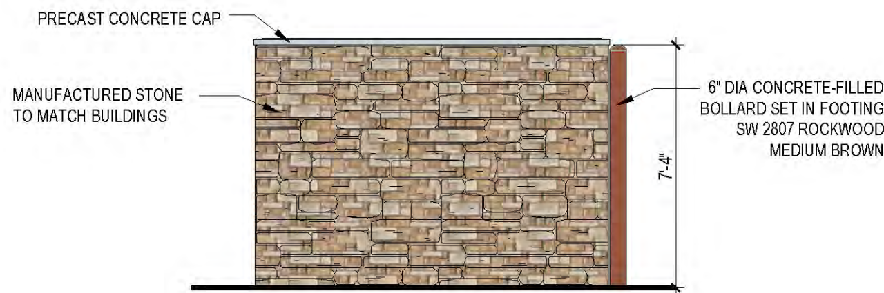
6 TRASH ENCLOSURE - SIDE ELEVATION 1/4" = 1'-0"
