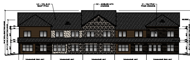
BLDG. TYPE VIB - SOUTH ELEVATION
