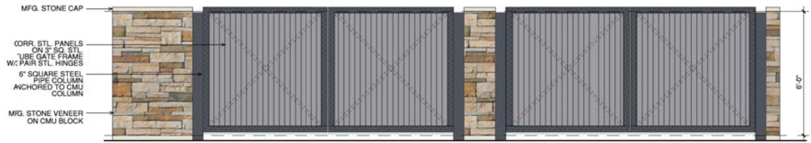
2 TRASH ENCLOSURE-FRONT ELEVATION SCALE: 1/2" = 1'-0"
