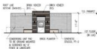
2 BUILDING 1 - EAST ELEVATION
