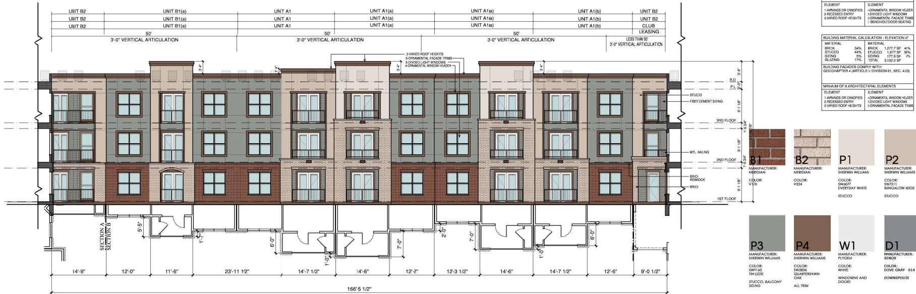
7 BUILDING A - COURTYARD ELEVATION
