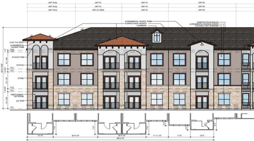
1b BUILDING - NORTH ELEVATION SCALE: 1/8" = 1'-0"
