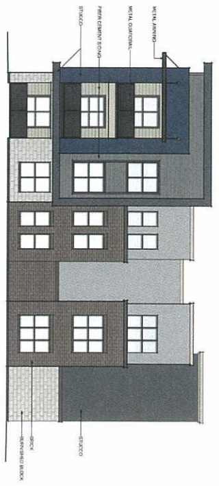
2 BUILDING 'A' ELEVATION - BLDG #5 & 6 NORTH SCALE: 1/8" = 1'-0"
