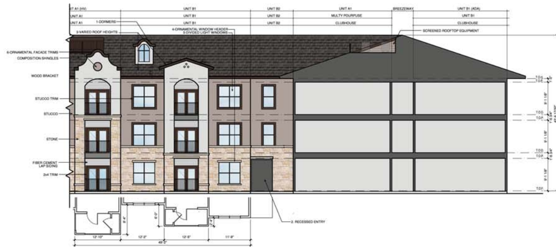
5a BUILDING - COURTYARD EAST ELEVATION SCALE: 1/8" = 1'-0"
