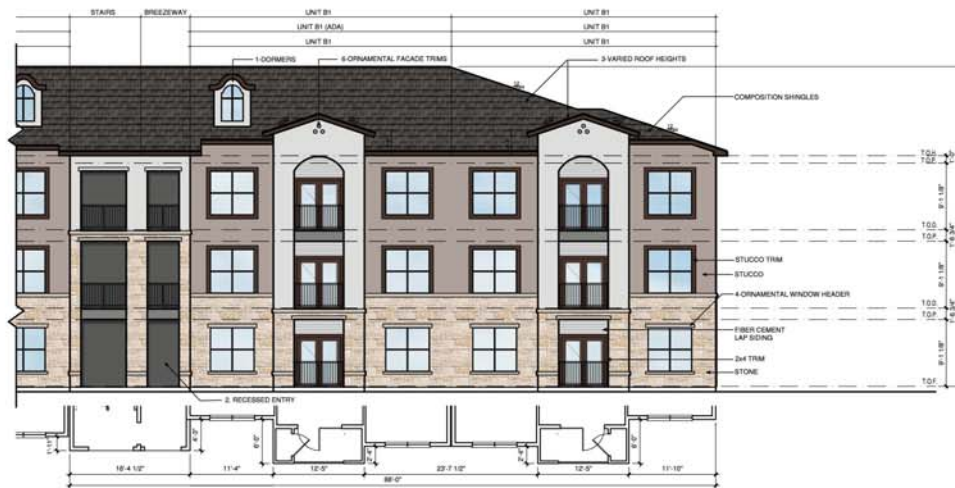
4b BUILDING - COURTYARD WEST ELEVATION SCALE: 1/8" = 1'-0"
