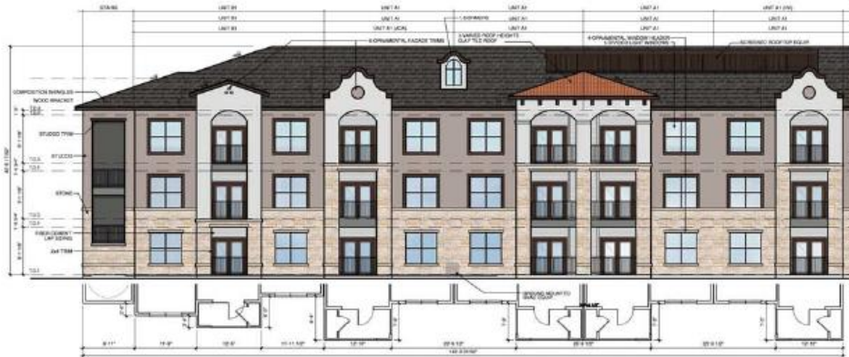
5a BUILDING - COURTYARD EAST ELEVATION SCALE: 1/8" = 1'-0"
