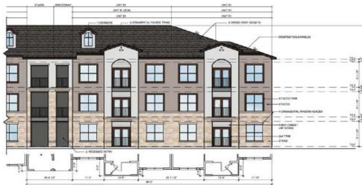
4b BUILDING - COURTYARD WEST ELEVATION SCALE: 1/8" = 1'-0"
