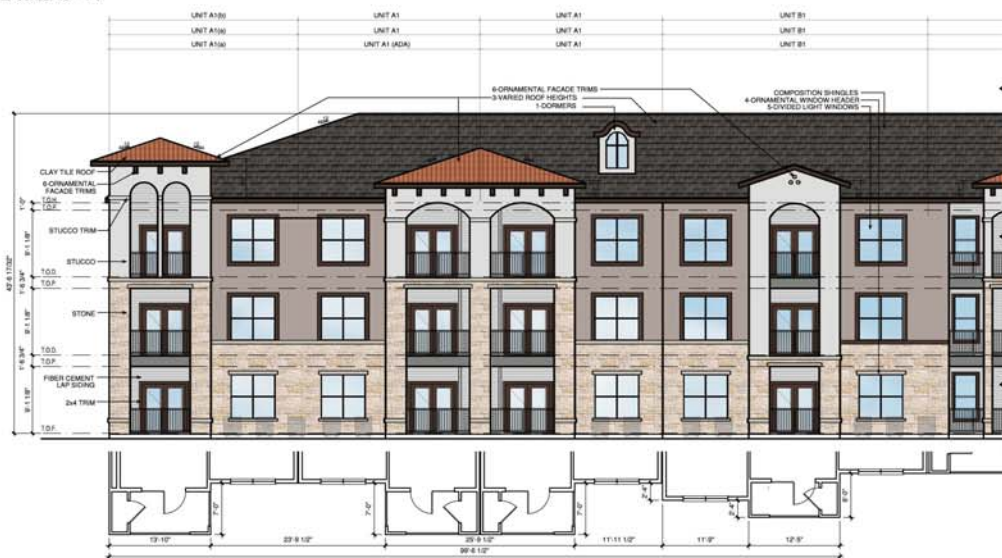
1b BUILDING - NORTH ELEVATION SCALE: 1/8" = 1'-0"
