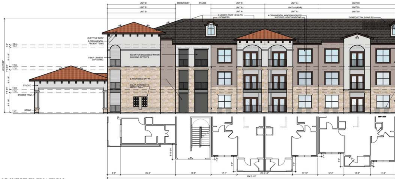
2a BUILDING WEST ELEVATION SCALE: 1/8" = 1'-0"
