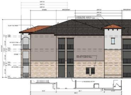
6a BUILDING - EAST ELEVATION SCALE: 1/8" = 1'-0"
