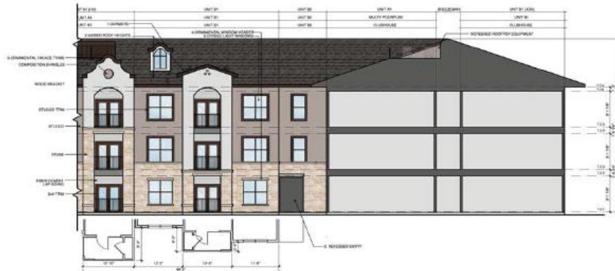
5a BUILDING - COURTYARD EAST ELEVATION SCALE: 1/8" = 1'-0"
