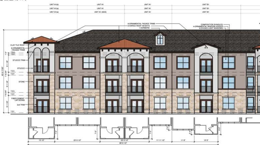
1b BUILDING - NORTH ELEVATION SCALE: 1/8" = 1'-0"
