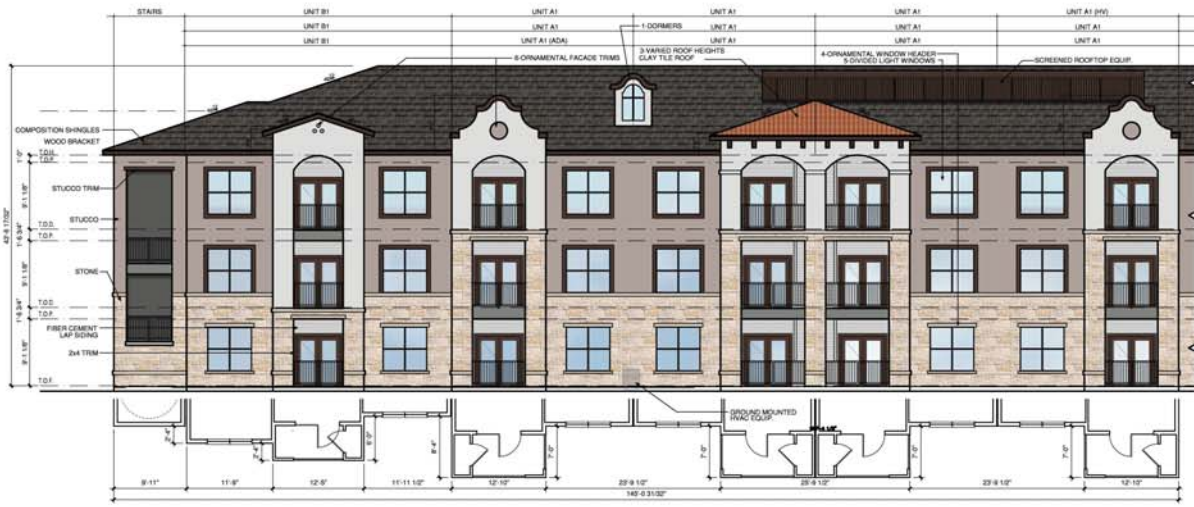
5a BUILDING - COURTYARD EAST ELEVATION SCALE: 1/8" = 1'-0"
