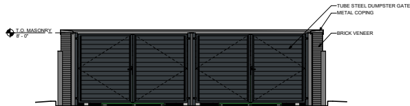
5 ELEVATION - DUMPSTER ENCLOSURE 1/4" = 1'-0"
