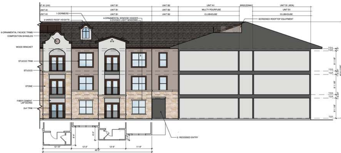
5a BUILDING - COURTYARD EAST ELEVATION SCALE: 1/8" = 1'-0"
