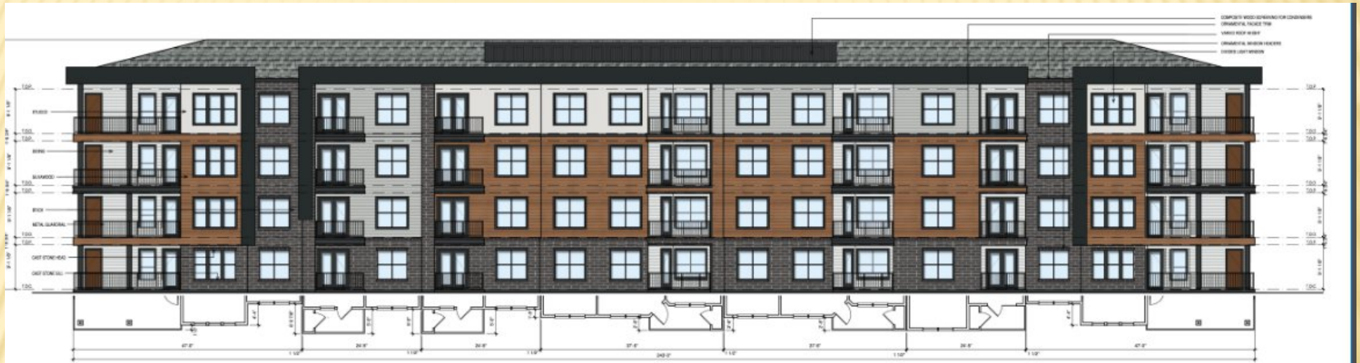
3 BUILDING TYPE 'B' ELEVATION
