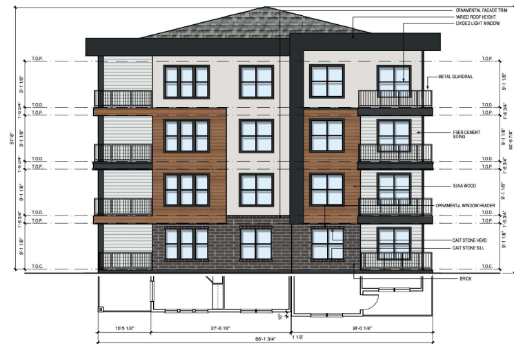
5 BUILDING TYPE 'A' ELEVATION
