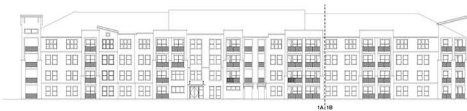
1 BUILDING 'C' SOUTH OVERALL ELEVATION SCALE: 1" = 20'-0"
