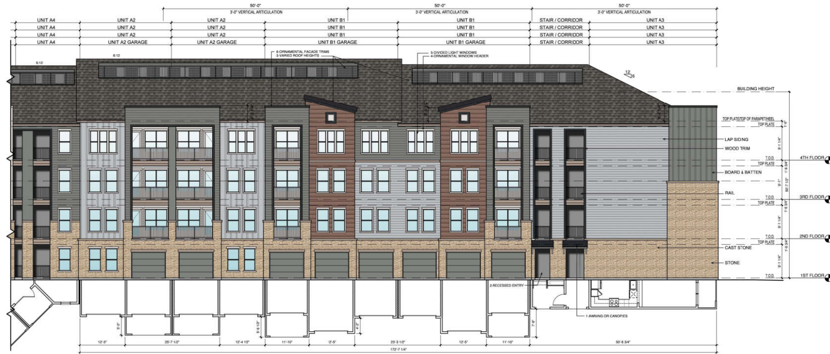
3b BUILDING B - NORTH EXTERIOR ELEVATION SCALE: 1/8" = 1'-0"
