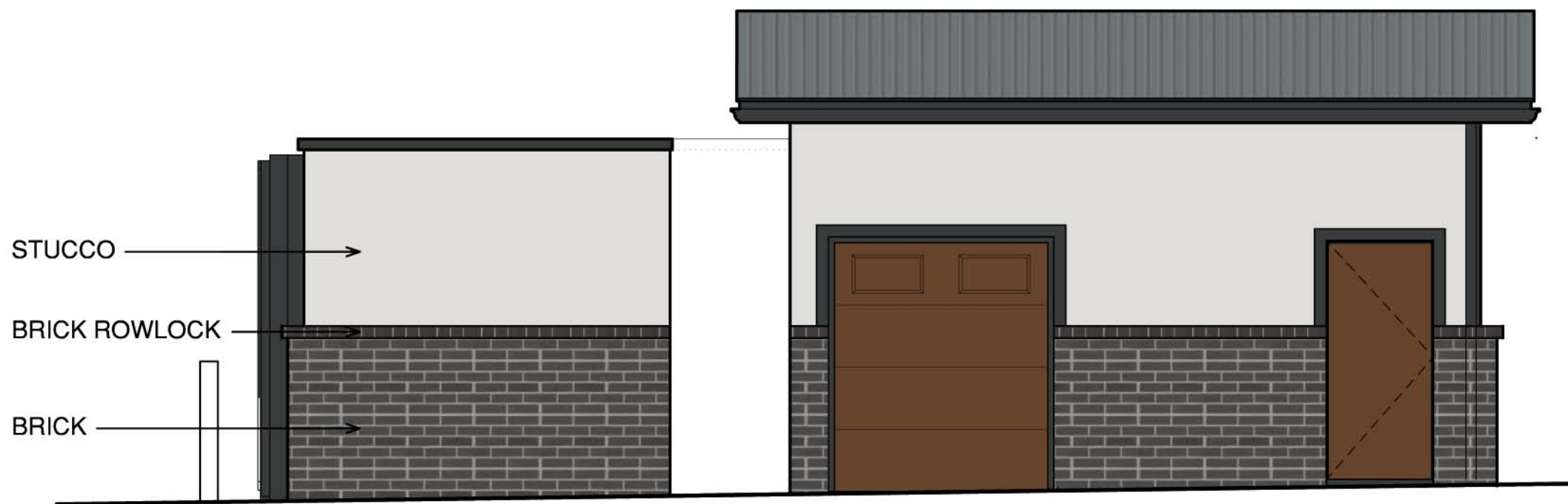
10 TRASH ENCLOSURE- WEST ELEVATION
