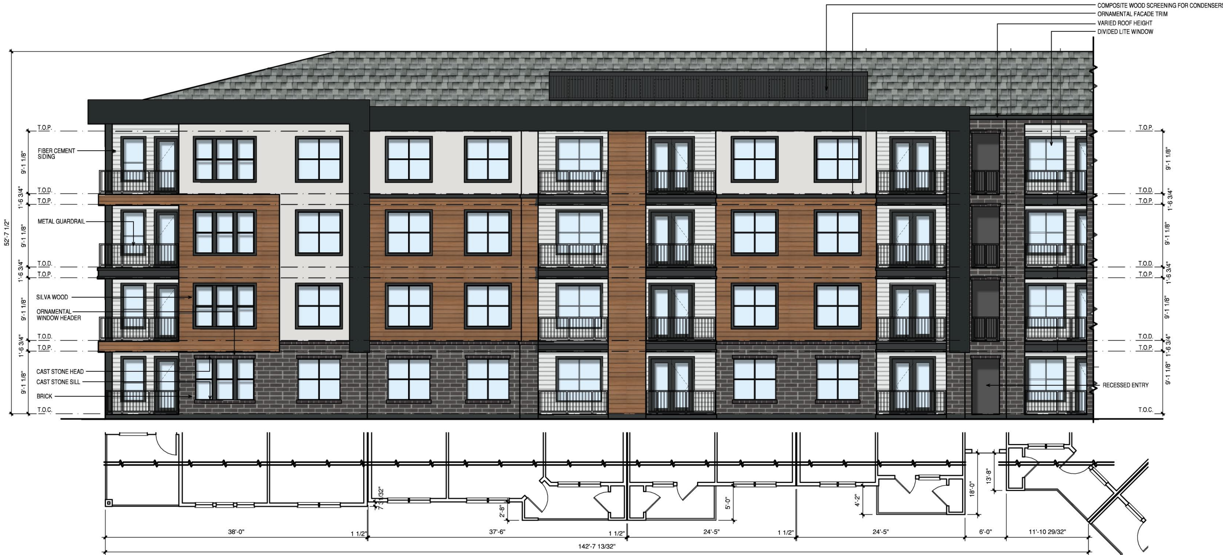
4 BUILDING TYPE 'C' ELEVATION
