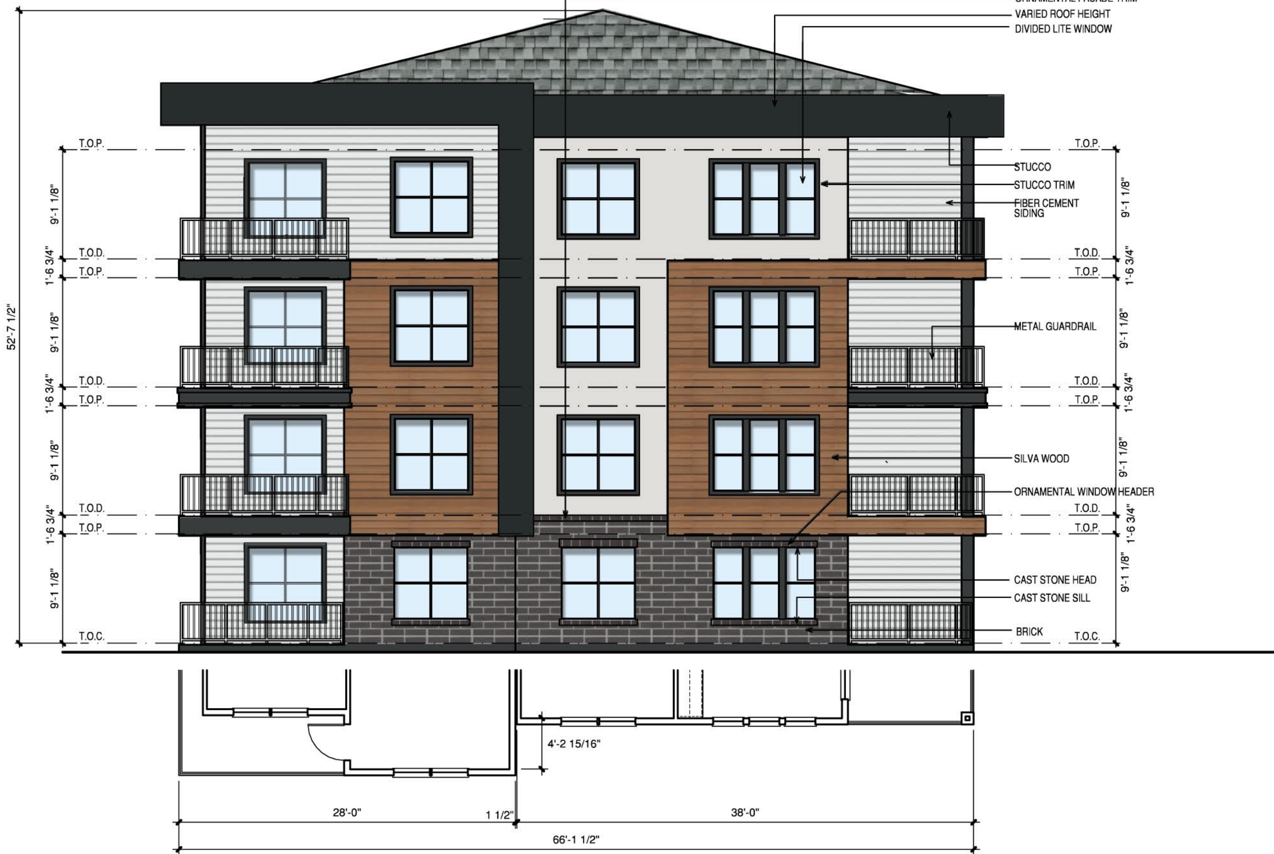
3 BUILDING TYPE 'C' ELEVATION
