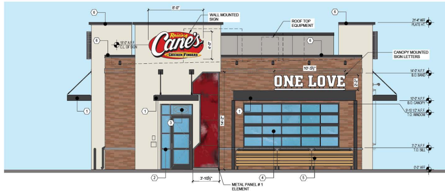
1 | NORTHWEST ELEVATION (FRONT ENTRY) SCALE: 1/4" = 1'-0"
