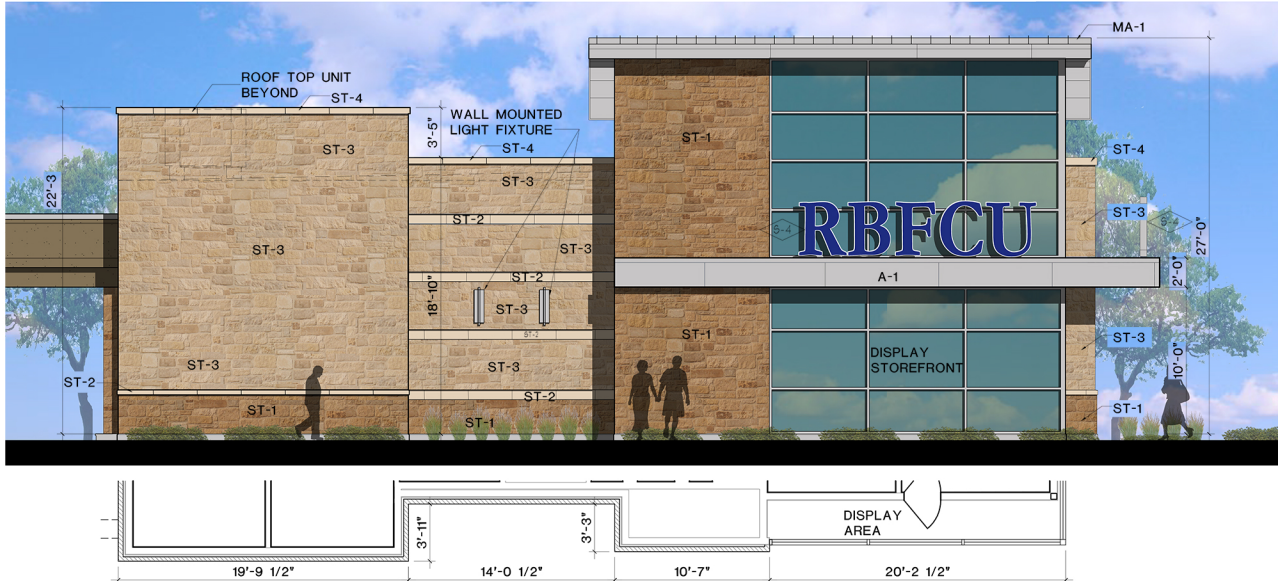
EAST ELEVATION (SIDE)
