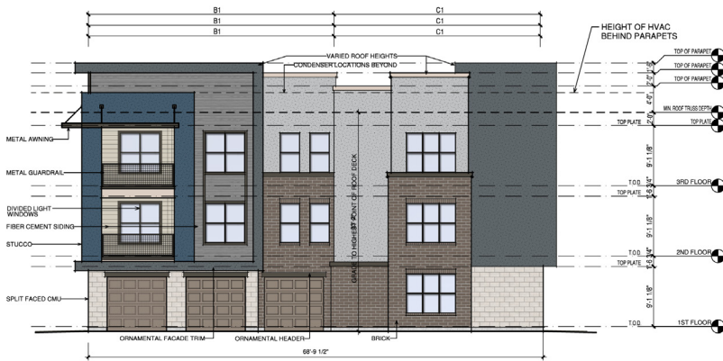
2 BUILDING 'A' ELEVATION - BLDG #2 SCALE: 1/8" = 1'-0"
