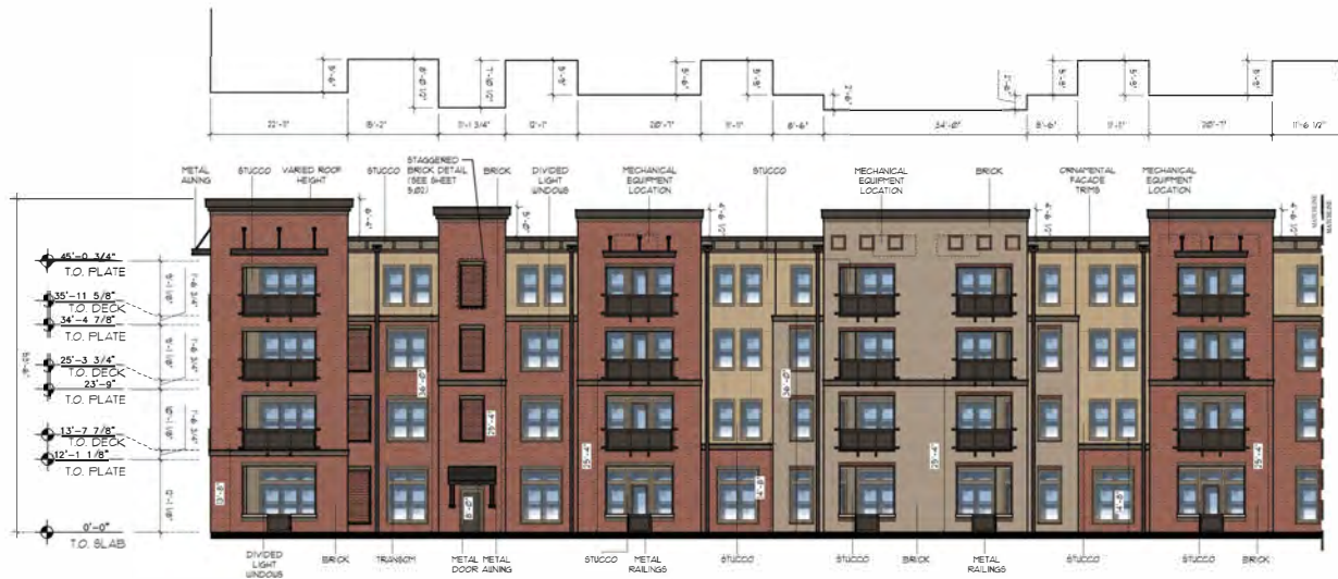
2 EXTERIOR ELEVATION (NORTH) SCALE 1/8" = 1'-0"
