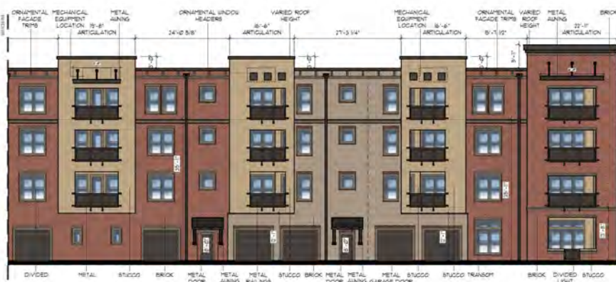
① EXTERIOR ELEVATION (WEST)
