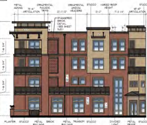
2 EXTERIOR ELEVATION (WEST)
