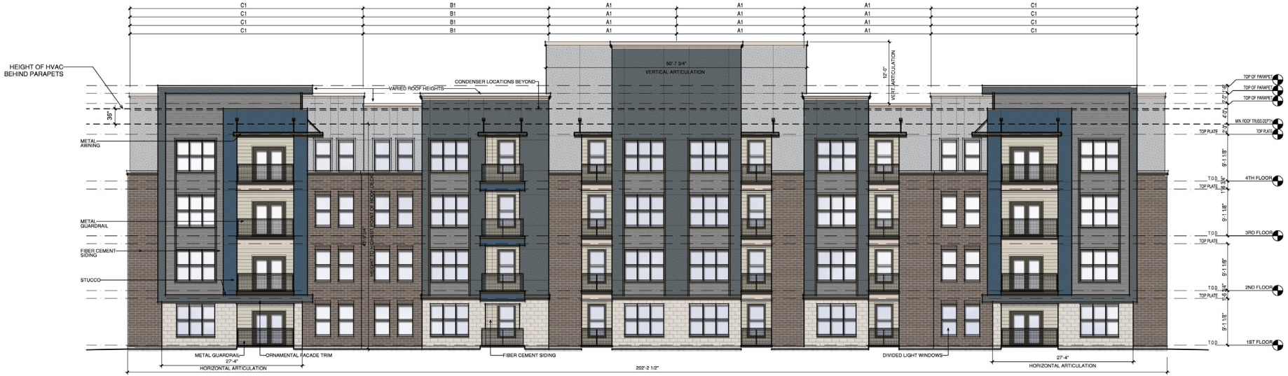
1 BUILDING 'B' ELEVATION - BLDG 1 SCALE: 1/8" = 1'-0"
