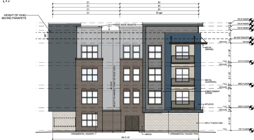
2 BUILDING 'B' ELEVATION - BLDG 1 SCALE: 1/8" = 1'-0"
