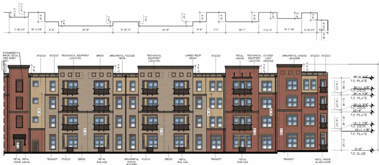
1 EXTERIOR ELEVATION (NORTH) SCALE: 1/8" = 1'-0"
