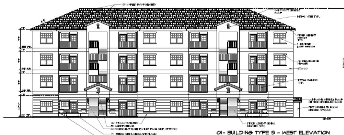
01- BUILDING TYPE 3 - WEST ELEVATION
