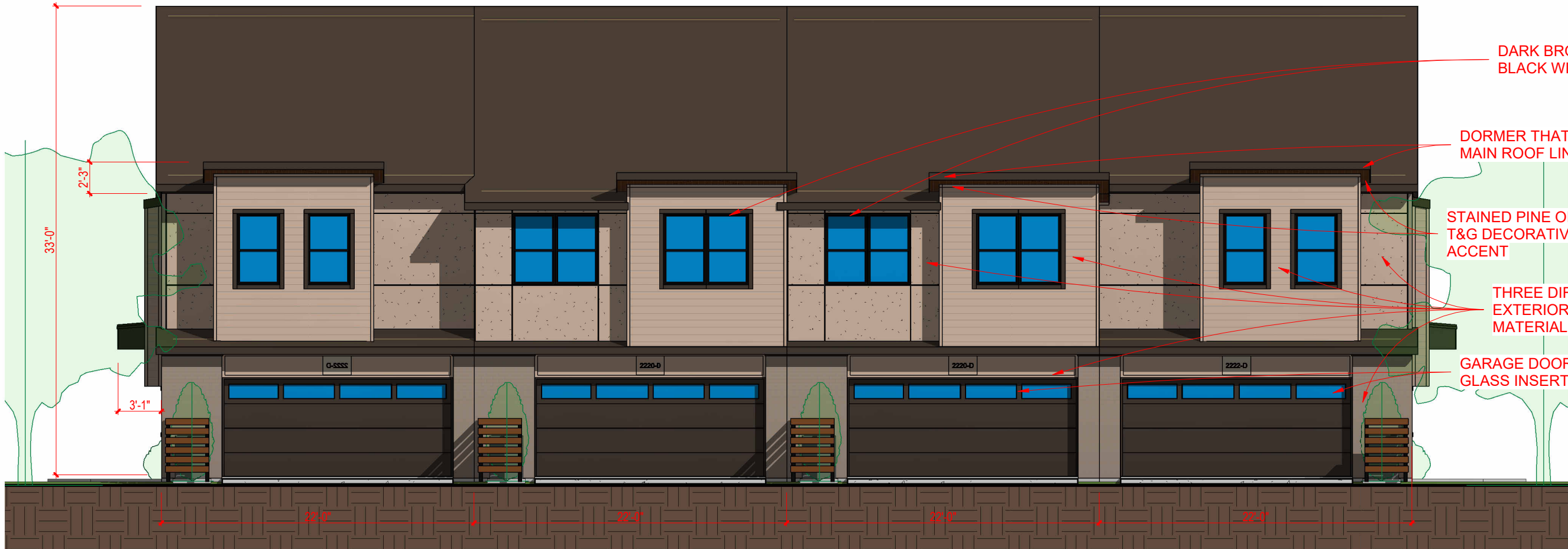
BUILDING STREET FRONT ELEVATION 1/8" = 1'-0"
