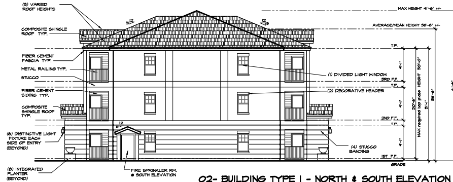
02- BUILDING TYPE I - NORTH & SOUTH ELEVATION
