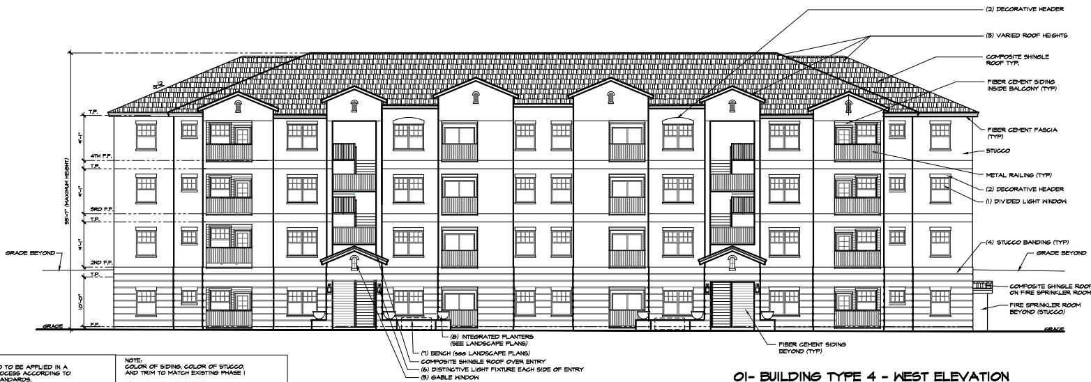
01- BUILDING TYPE 4 - WEST ELEVATION
