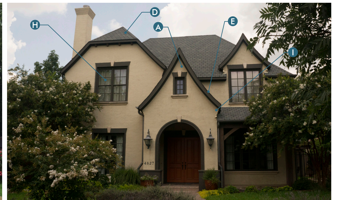
A Prominent front facing cross gable; B Nested gables; C Asymmetrical eaves; D Clipped gable; E Sweeping eave; F Shed dormer; G Decorative half-timbering; H Ganged windows; I Brick corbels
