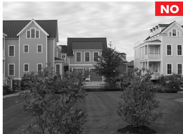
Garage is inappropriately placed with the garage doors orienting onto a common space and terminating a view corridor.
